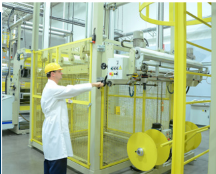
Operator moves the blade assemblies into the desired position by rotating the mechanism hand wheels
