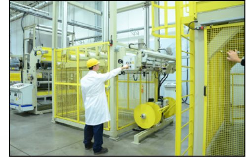
Operator shuts off accumulator to deactivate the safety cage door lock for access purposes
