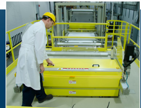
Operator accesses guard hatch door to the driven nip rolls on top of the mezzanine
