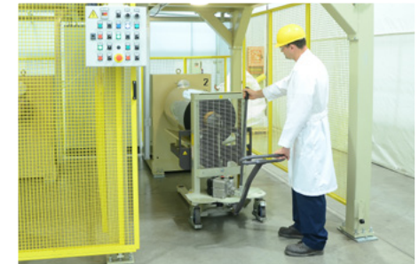
4. Cart cradle is raised using the hydraulic hand pump (right hand) until the roll weight is fully supported
