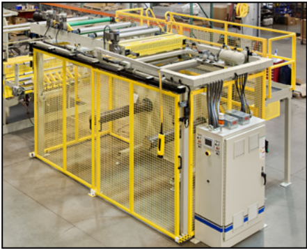
Model CW-5440/2 Cantilever Winder featuring 2 winding positions and full surround safety caging
