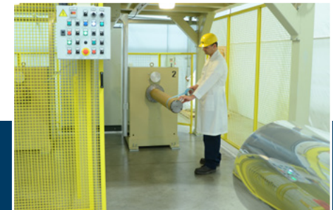
8. Transfer prep is completed once double-sided tape is applied to the new core & core rod shaft is re-inflated
