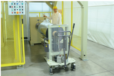
5. Pneumatic push-off mechanism (lever controlled) is extended until the roll travels off the spindle
