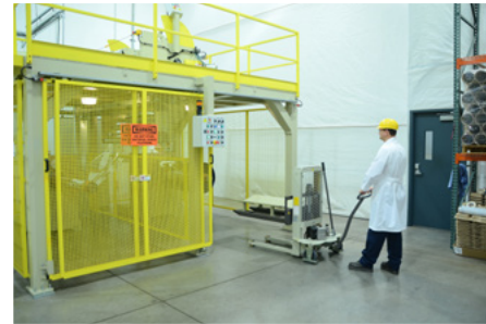
3. Roll removal cart is centered under the wound roll into the proper unloading position
