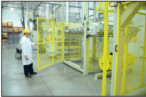
Operator gains access thru safety cage door during maintenance and web-up activities
