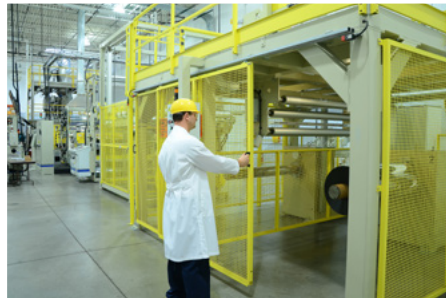
2. Safety door is opened to initiate wound roll removal & the core rod is deflated
