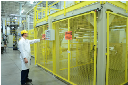
1. Transfer completed from the prior steps shown & the safety door is unarmed for access
