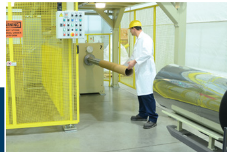
7. A new winding core is inserted onto the core rod shaft
