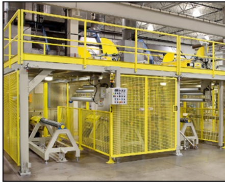
A-Frame Winder Model AW-7248/4 has 4 winding positions at 72 in. widths & 48 in. roll diameters
